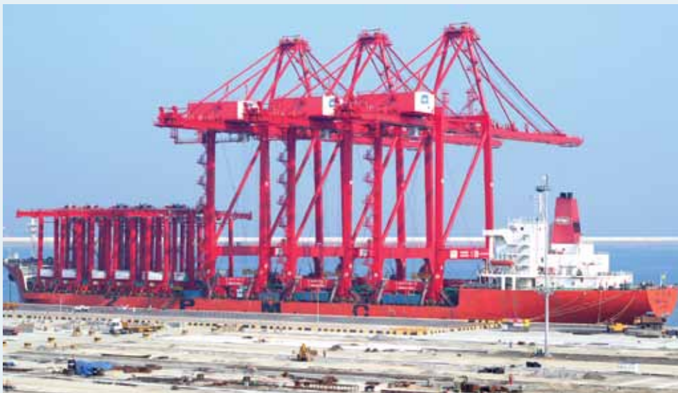
ZPMC Company Lanka unloading ship to shore gantry cranes at Colombo International Container Terminal, Port of Colombo
